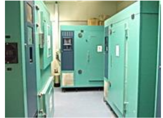
Plant Growth Chamber
